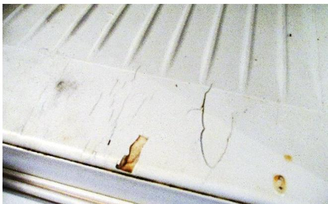
**The damage to the lining in this refrigerator is so extensive, the cost to repair the broken parts was more than a brand-new unit.** Replace refrigerator from misuse: \$400.00
