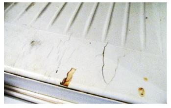
The damage to the lining in this refrigerator is so extensive, the cost to repair the broken parts was more than a brand-new unit.
